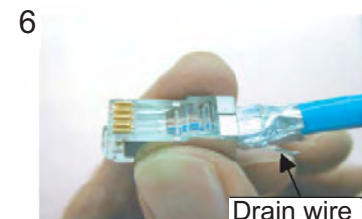
6 Insert the cable into the modular plug so that the folded part of the shield enters into the plug housing. The drain wire should be located on the tab side of the jack.
